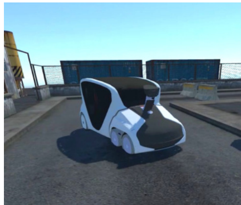
Figure 2: The VR Lab: a scenario consisting of the CityBot base module (tractor) with the small taxi module attached.
